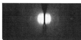
Fig. 5. A line-focus low-angle X-ray diffraction pattern of rat sciatic nerve in Krebs-Ringer's solution. The pattern was taken using 30 kV copper K\alpha nickel-filtered radiation, a specimen-to-film distance of 5.5 cm, an exposure time of 12 h and the radial period was d = 176 Å. The central region is over-exposed in order to show the higher orders of diffraction. Diffraction orders h = 3, 4, 5, 6, 8 , and 11 are clearly visible while weaker orders h = 7, 10 are just discernible.
